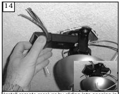
Install remote receiver by sliding into opening in the Mounting bracket. Make sure that the dip switches on the Transmitter and the Receiver are set to the same position. See Fig 31 for remote operation
